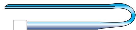
Minimum bend radius of fiber is 0.062". Actual cable bend radius may be greater.
